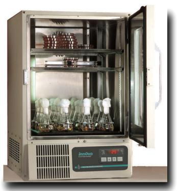
**Front-loading Innova 4200 & 4230 shakers** accept a wide variety of interchangeable  $18" \times 18"$  (46 x 46 cm) accessory platforms for glassware up to 6 liters. Two stationary shelves are included for incubating or refrigerating added samples.
